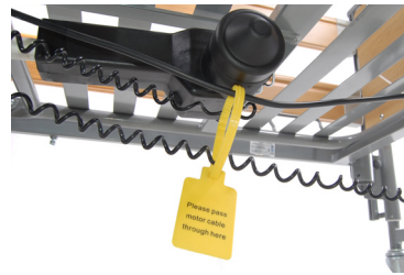
The foot actuator cable MUST go through the yellow cable tie. Wrap the actuator cable round the power cable to reduce the amount of hanging wires under the bed.
